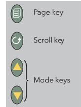
After Set2 parameters have been edited, a further operation of the scroll key invites the user to Exit. Operating the scroll key returns to the Set1 display; operating a mode key to display 'yes' quits the quickstart menu and causes the unit to enter operating mode.
