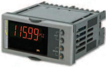
Model number 32h8e is a horizontal 1/8DIN indicator and alarm unit that performs the dual function of remote display for EPower and independent 'policeman'. The latter is intended to disconnect should an overtemperature (or other excess process condition) occur.
