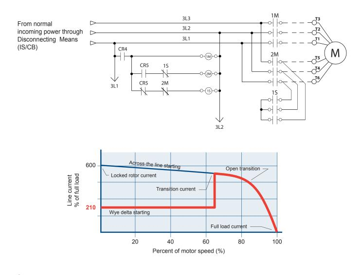
Starting Method: Reduced Voltage Wye-delta open Typical Voltage Applied at Start: 100% Inrush Current: 33% of normal load current Starting Torque: 33% Motor Type: Wye-delta No. of Contactors: 2 at 58%, 1 at 33% of motor full load current (FLC) Min. ampacity of motor conductors: 6 at 125% x 58% of FLC
