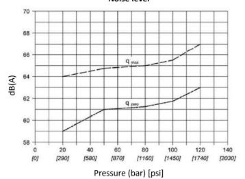
Indicative maximum noise level values measured with sound-level meter placed one metre [39.370"] from the pump, with flexible coupling
